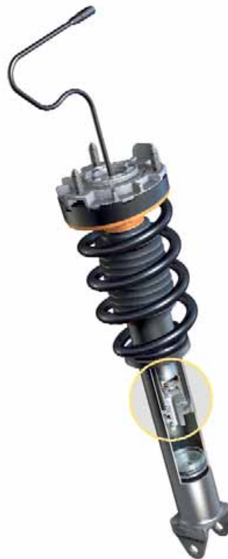
Rebound in 'Normal' mode – damper piston with bypass valve open
