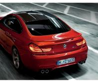
Technology taken directly from the track: the M6 Coupe's carbon fiber roof. It optimizes aerodynamic airflow, while its lighter weight lowers the car's center of gravity to enhance cornering and agility. Exceptionally rigid and sturdy, it adds to the M6's handsome looks, too.
