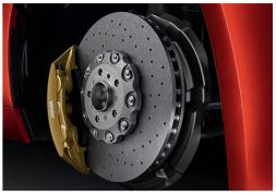
M Carbon Ceramic Brakes in the BMW M6 Coupe and Convertible have an extremely high load capacity and excellent resistance to fade. The system can be identified by the gold brake calipers with M logo.
