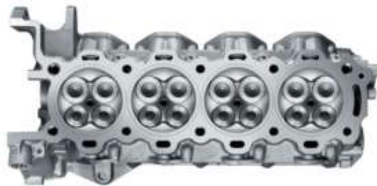
Motore F430: testata 8 cilindri in alluminio The 4-valve head of the F430's V8
