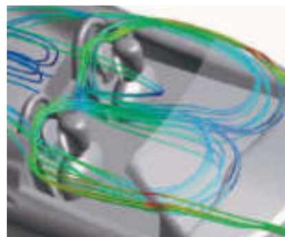
Andamento delle linee di flusso in abitacolo Computer simulation of the air flow in and around the passenger.
