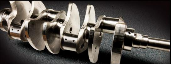
"This is essentially an all-new powertrain that's unique to GT350, and it takes full advantage of the new Mustang platform's outstanding chassis dynamics. Make no mistake, the engine is an American interpretation of a V8 with flatplane crankshaft, and it produces a distinctive, throaty how! from its four exhaust tips."
