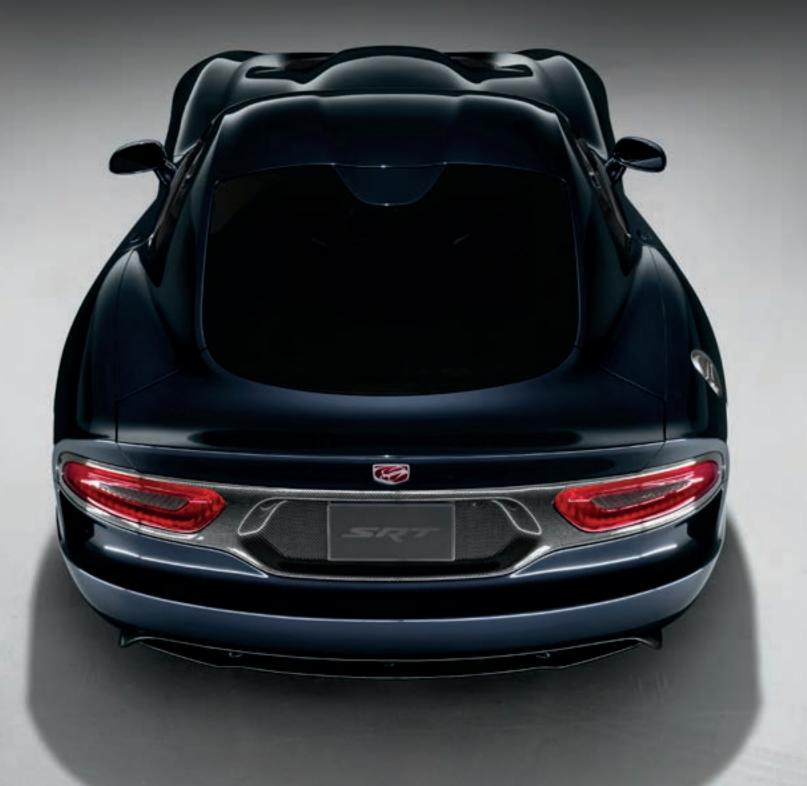
down and performance rates up. The hood itself resurrects the popular clamshell design and, along with the roof and deck-lid, is designed with all-new carbon fiber construction for significant weight savings.
